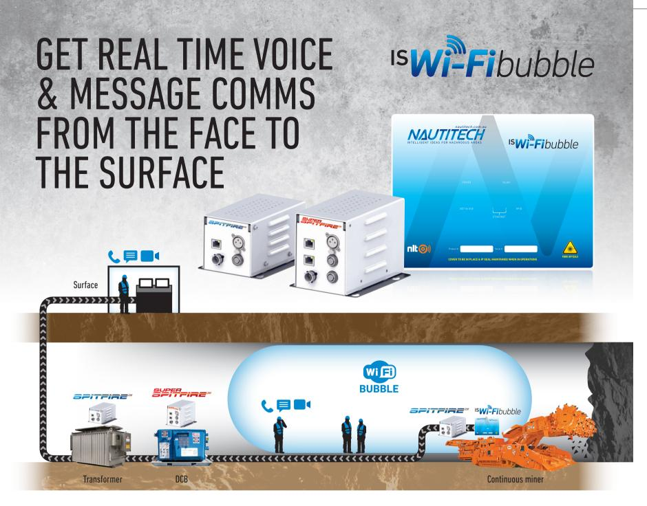
General communications and the reporting of incidents occurring around the coal face has traditionally been hampered by the need for mine employees to physically walk back to the crib room and pick up the phone in order to make requests such as for parts or emergency help. A new combination of powerline modem and Wi-Fi comms technology solves this communication lag that can often come at a critical time, by enabling immediate comms from the face.
